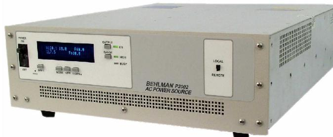
The new Behlman 2 KVA Power Source provides clean, regulated AC power at operator selectable voltage from 0 - 135 or 0 - 270 VAC, and adjustable frequency from 45 - 500 Hz, in a single 5.25" high bench-top chassis that easily converts into a rack mount unit.
